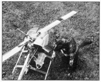
fuel proofing and painting everything was fitted to chassis and servos fitted. The linkages were then made up to exact lengths given, no difficulties
